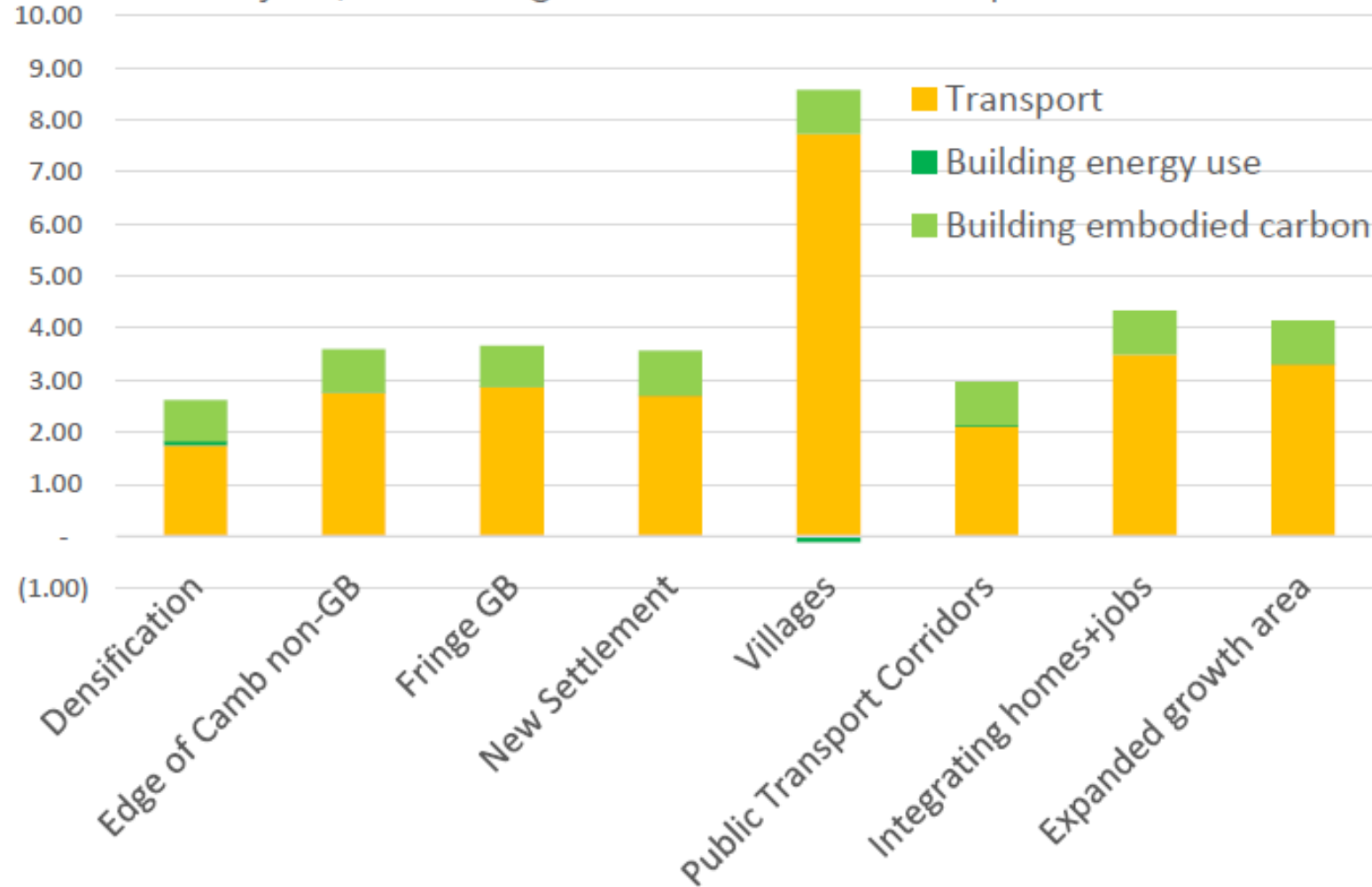
Figure 3: Per home annual emissions (tCO 2 ) for 2030 (mid plan year), medium growth, with zero carbon policies
