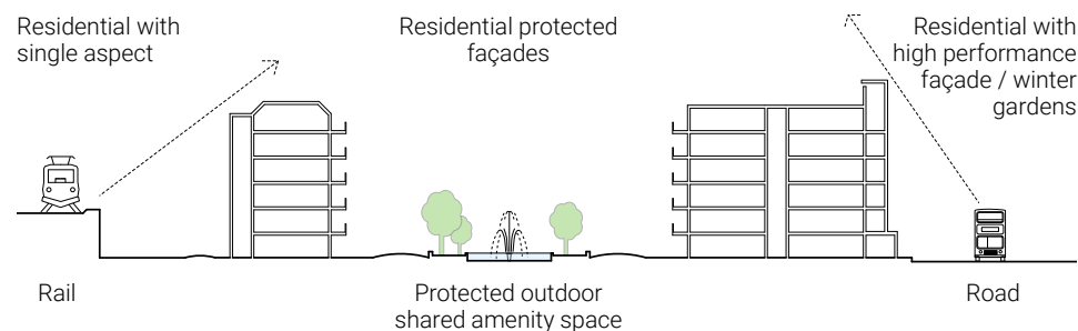
Figure 5. Noise mitigation measures through landscaping, site and building layout: noise from rail and road is buffered by the taller buildings, protecting the dwellings and landscaped areas on the other side (provided by Studio Partington).
