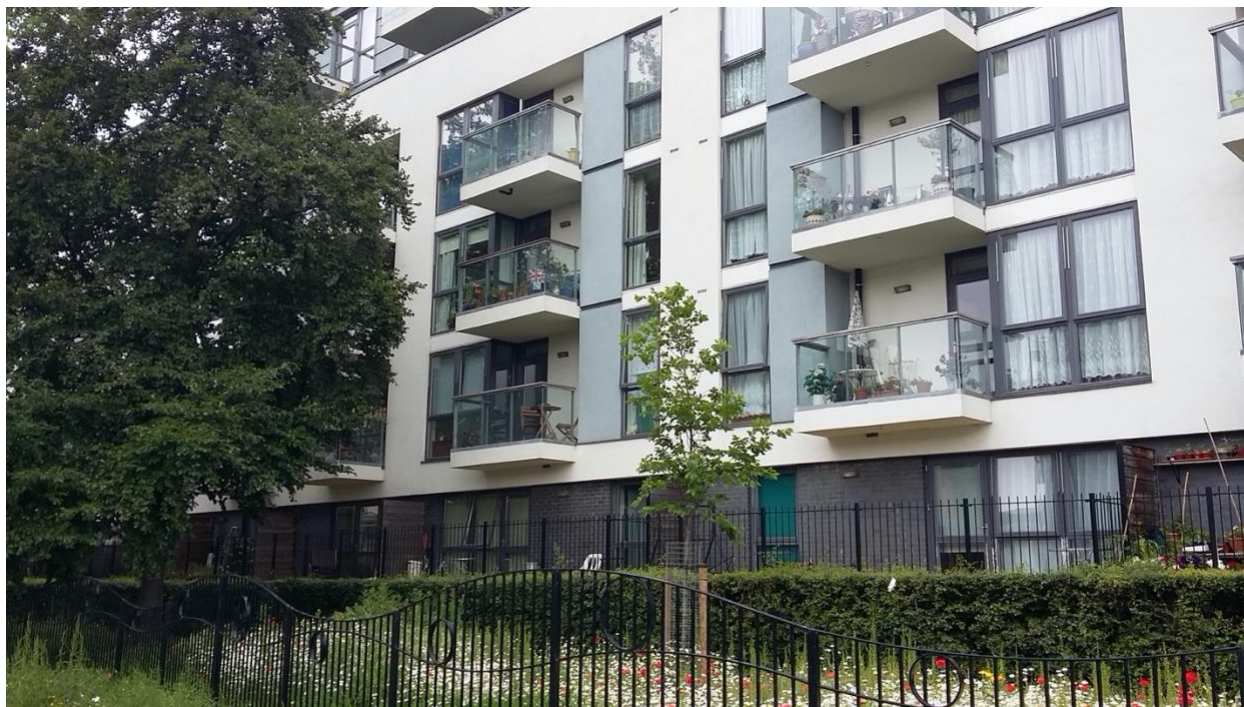
Figure 20: The large mature tree on the left provides substantial shading to dwellings immediately behind it, which may even warrant extra mitigation points under question #14. This shading is only available to part of the building: the nearby tree, on the other hand, is still very young, producing hardly any shade: it should not be taken into account, unless possibly to test future scenarios. Scoring for the block should not account for trees, unless if scoring specifically for the shaded dwellings.
