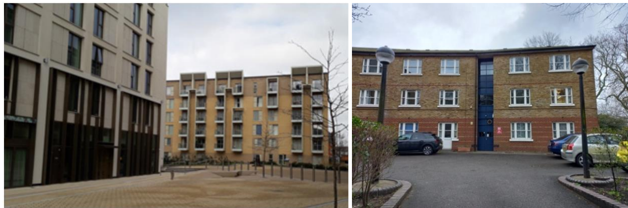
Figure 17: Example of light-coloured (high albedo) facades and external hard surfaces (left) and tarmac (right). Ground surface temperatures are likely to be lower in the left-hand example than the right with a consequent impact on local air temperatures in hot weather, for a given similar location
