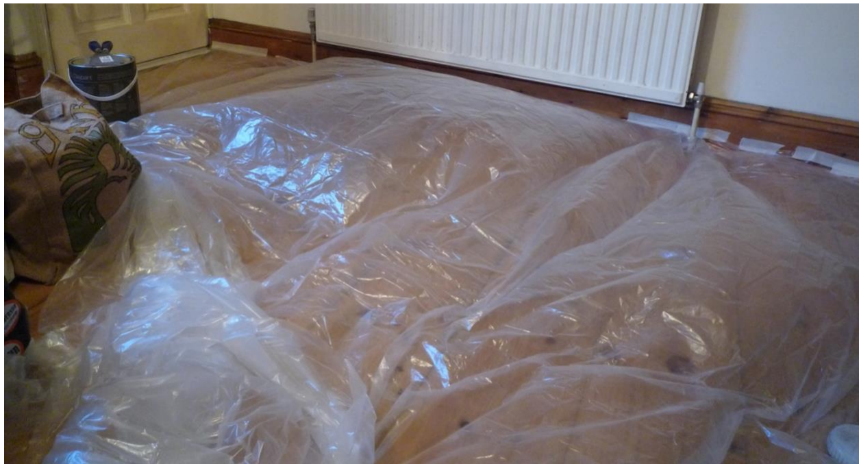
Figure 44: Suspended timber floors can be a significant leak feature, as illustrated by this plastic sheet covering the floor during works, blown from air rising from beneath
