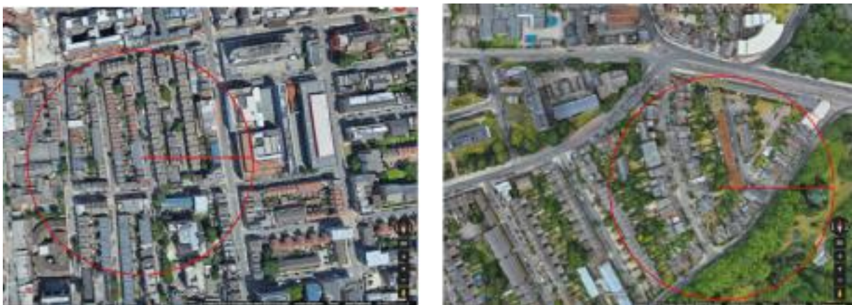
Figure 10: Examples of using satellite view (google) to help score this question: these two sites in East London have similar built typologies with mostly low-rise housing and some isolated high-rise blocks and would score the same for overall urban heat island effect (#2) because of their location in Tower Hamlets and Hackney. However, at the local scale (100m radius) they have very different characteristics in terms of green infrastructure, with the left-hand side site likely to experience higher local temperatures
