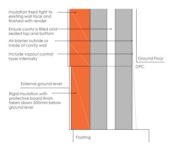
Figure C.9 - Insulation strategy for cavity wall - external wall insulation (EWI)
