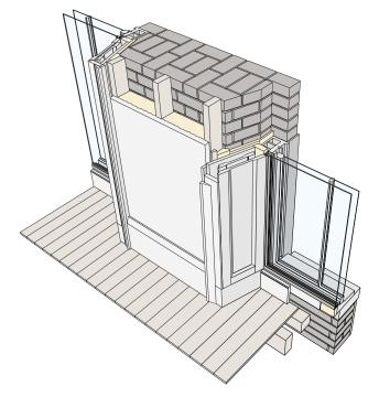
Figure 6.30 - Axonometric showing insulation to walls, shutter box and secondary glazing to existing windows, Prewett Bizley Architects
