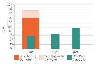
Figure 1.11 - Gas heating demand and gas hot water demand compared to electrical grid peak capacity.
