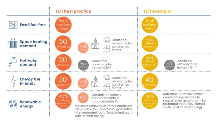
Figure 4.1 - LETI retrofit energy targets. Figures given in kWh/m²/year (treated floor area or 90% of gross internal floor area)
