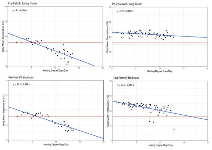
**Figure 6.15** - Scatter plots show a single dwelling (living room and bedroom) that are under-heated prior to the retrofit, and currently maintains significantly better internal temperatures utilising the same heating practice post retrofit<sup>6.6</sup>.
