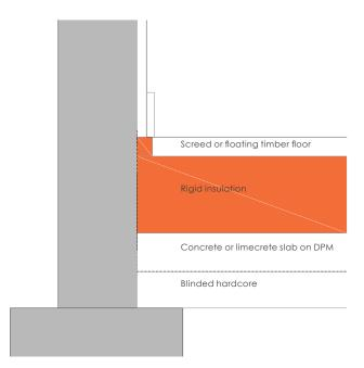
Figure C.7 - Insulation strategy for removed suspended timber floor
