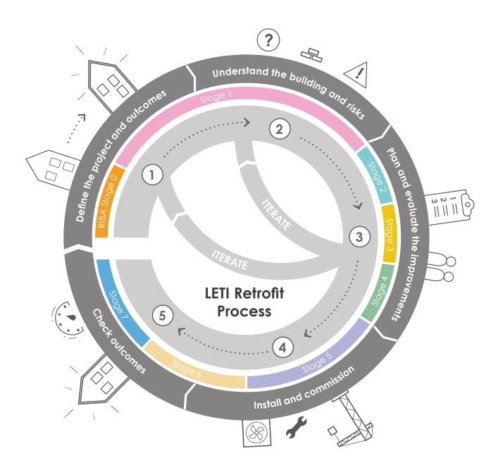
Figure 5.3 - LETI Retrofit Process summary diagram showing the key stages and how, where necessary, early design and evaluation gives a chance to revisit the project definition and building evaluation with new information.
