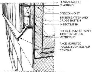
AXONOMETRIC VIEW DETAIL - REAR EXTENSION
