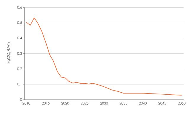
Figure 2.5 - Decarbonisation of the electricity grid.
