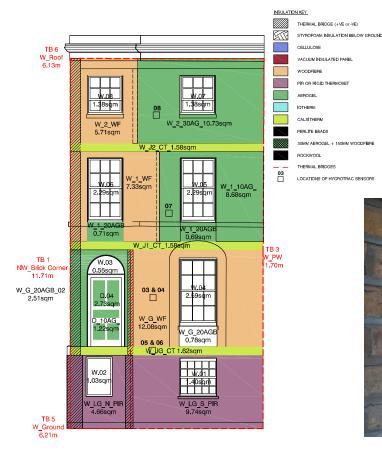
Figure  ${\bf 6.39}$  - Schematic of types of insulation to rear elevation, Arboreal Architecture
