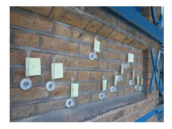
Figure 6.40 - Hygrothermal monitors between existing masonry walls and new internal insulation, Arboreal Architecture
