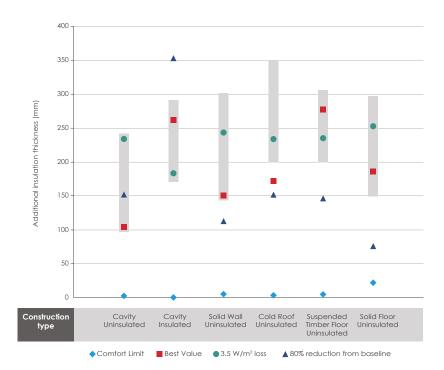
Figure G.6 - Thickness of additional insulation by baseline construction (ext temp -5 Degrees Celsius)
