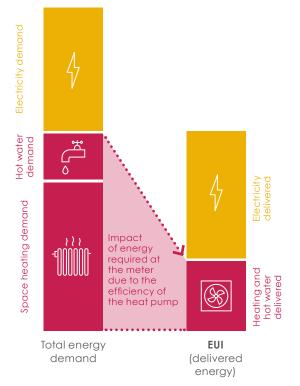
Figure  ${\bf 3.4}$  - Relationship between energy demand and EUI when using a heat pump.
