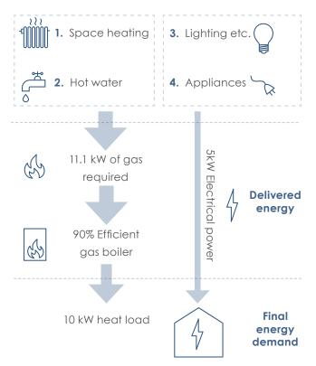
Figure A.1 - Delivered and final energy for 90% efficient gas boiler
