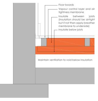
Figure C.5 - Insulation strategy for retained suspended timber floor
