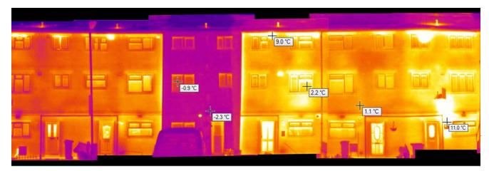
Figure 6.28 - Thermal imaging winter 2012 post retrofit, bere:architects
