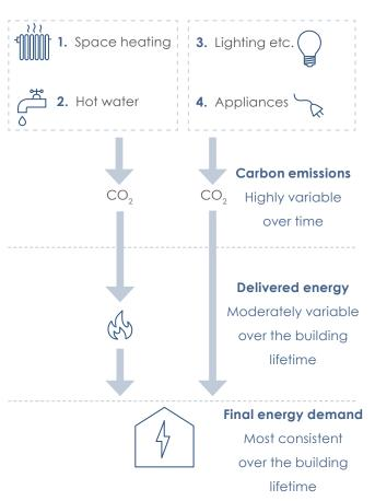
Figure A.4 - How variable is the chain of delivery of energy to the building
