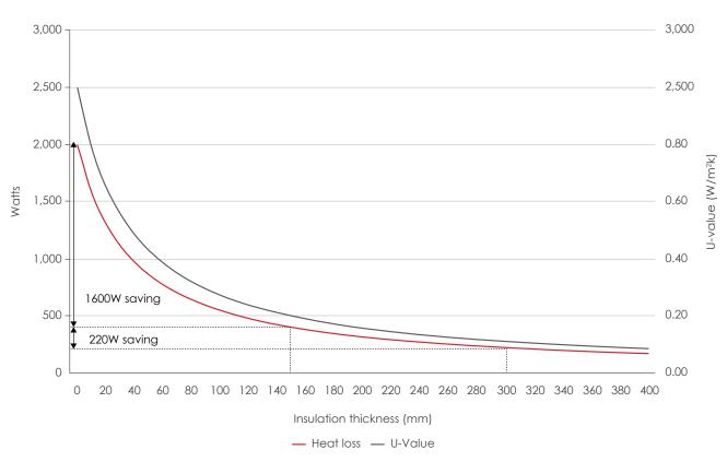
Figure G.1 - Diminishing returns for the amount of insulation being applied to a  $100m^2$  solid wall with external temperatures at  $0^\circ\text{C}$
