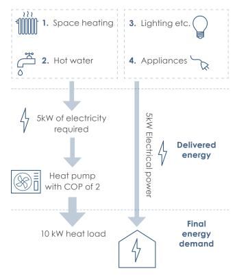
Figure A.2 - Delivered and final energy for heat pump with COP of 2
