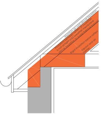
Figure C.12 - Insulation strategy for cold roof insulated between and above ceiling joists
