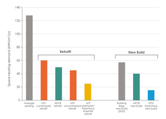
Figure 3.15 - Space heating demand comparison <sup>3.5</sup> (LETI retrofit cases highlighted in orange).
