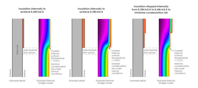
Modelling parameters: 0°C externally, 20°C internally. Brick conductivity 0.77W/m.K; insulation conductivity, 0.04W/m.K
