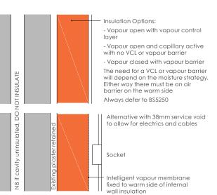
Figure C.11 - Insulation strategy for cavity wall - internal wall insulation (IWI)
