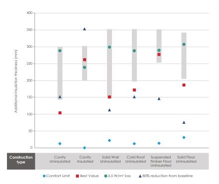
Figure G.8 - Thickness of additional insulation by baseline construction (ext temp -10 Degrees Celsius)
