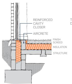
**OPTION 2** INSULATION AT DOOR THRESHOLD
