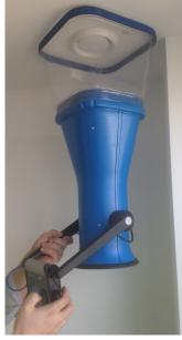
MEASURE AIRFLOW WITH APPROPRIATE DEVICE
