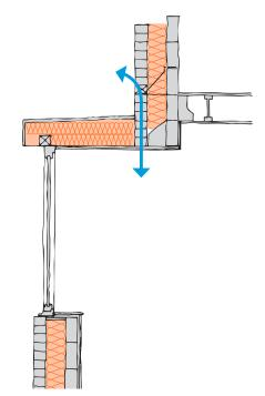
THICK FRAME AND POSTS INCREASES HEAT LOSS
