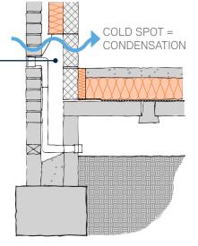
PLAN OF SUB FLOOR VENT BLOCKING INSULATION
