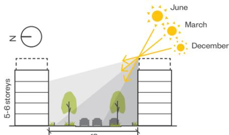
Avoid overshadowing of buildings, this reduces the heat gain from the sun in winter. Allow 1-1.5m of distance for every 1m of height.
