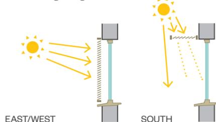
East/west orientations have a higher overheating risk due to low-angle sun. Reduce glazed areas and include shading on the west, e.g. with shutters.
